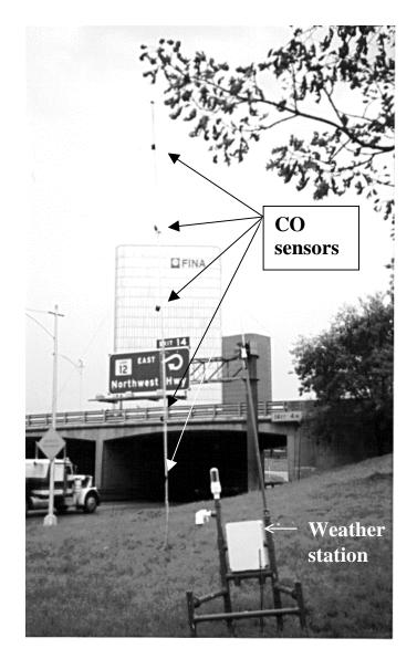
Figure 14. Vertical Placement of CO Sensors and Weather Station for a Depressed Freeway (Site: Dallas, near Intersection of Loop 12 and U.S. 75)
