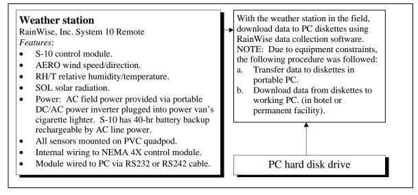
Figure 18. Meteorological Data Transfer Procedure
