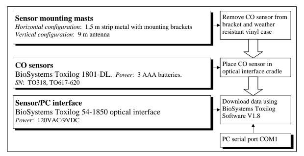
Figure 17. CO Data Transfer Procedure
