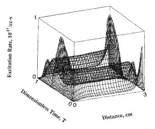
FIG. 15. Spatial and temporal variation of the excitation rate for the electronegative discharge. Conditions were at their basic value.
