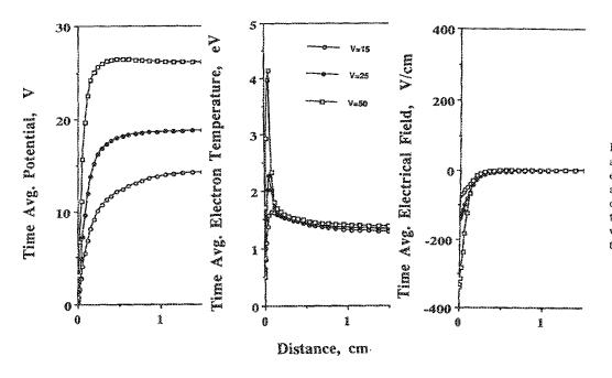
FIG. 7. Spatial and temporal variation of potential time-average electron temperature and timeaverage electric field as a function of position in the gap for the electropositive discharge. Conditions were at their basic value except for the applied rf voltage.
