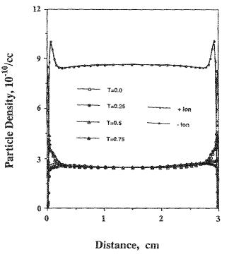
FIG. 9. Spatial and temporal variation of electron, positive ion, and negative ion density for the electronegative discharge. Condition were at their basic value. The electron density has been multiplied by 100.
