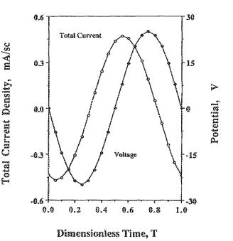
FIG. 4. Total current and voltage waveforms for the electropositive discharge. Conditions were at their basic value.
