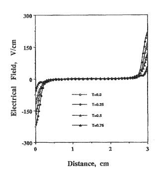
FIG. 3. Spatial and temporal variation of the electric field for the electropositive discharge. Conditions were at their basic value.
