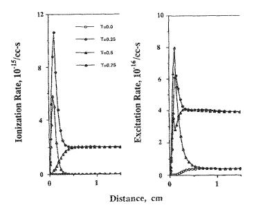
FIG. 13. Spatial and temporal variation of the ionization rate and excitation rate for the electronegative discharge. Conditions were at their basic value.
