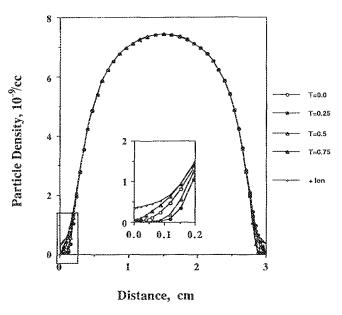
FIG. 1. Spatial and temporal variation of electron and positive ion density for the electropositive discharge. Conditions were at their basic value. Inset shows an expanded view of the sheath region.
