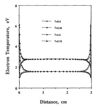
FIG. 12. Spatial and temporal variation of the electron temperature for the electronegative discharge. Conditions were at their basic value.
