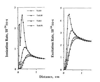
FIG. 6. Spatial and temporal variation of the ionization rate and excitation rate for the electropositive discharge. Conditions were at their basic value.
