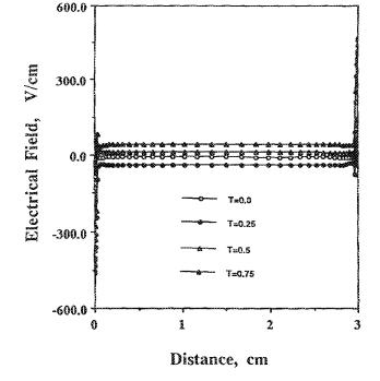
FIG. 11. Spatial and temporal variation of the electric field for the electronegative discharge. Conditions were at their basic value.
