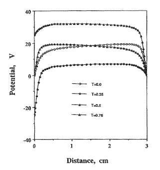
FIG. 2. Spatial and temporal variation of the potential for the electropositive discharge. Conditions were at their basic value.
