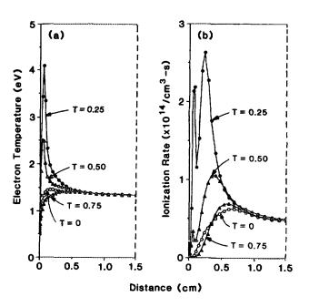
FIG. 2. Spatial and temporal variation of electron temperature (a) and ionization rate (b) for a pressure of 1 Torr.
