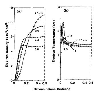
FIG. 3. Time-averaged electron density (a) and electron temperature (b) in the gap for different spacings. Pressure was 1 Torr.
