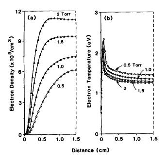
FIG. 1. Time-averaged electron density (a) and electron temperature (b) in the gap for different pressures.
